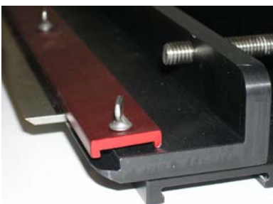
Carriage with knife in clamp
